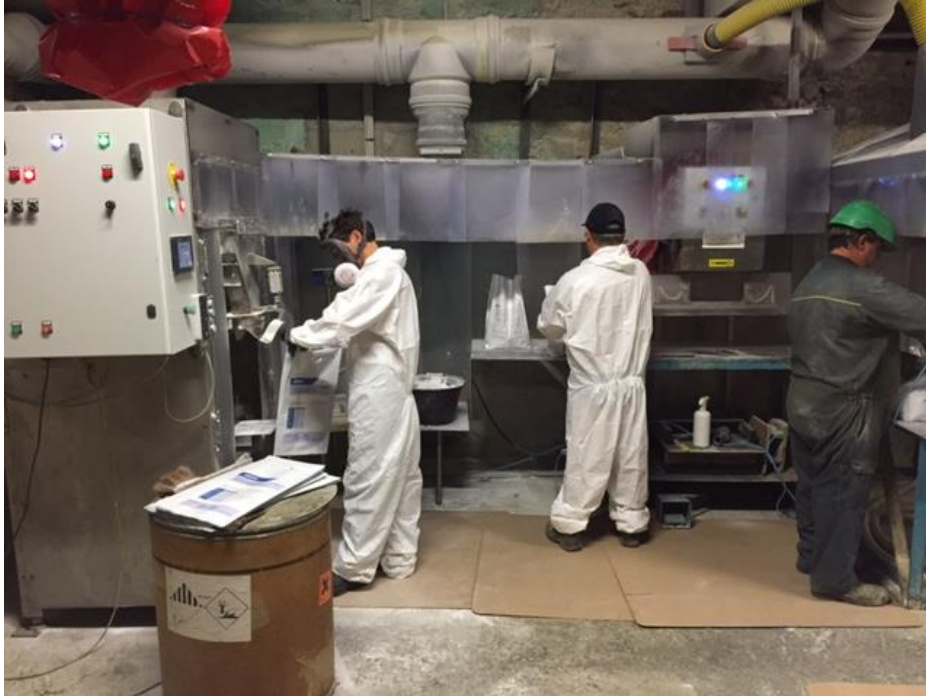
Packaging line composed of an automatic bagger and a welder
